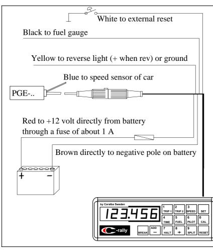
Make sure all connections are done professionally. The cables should be fixed avoid to damage. Most disturbances in function that occur are caused by poor connections to the power supply. After having carried out these functions simply connect each part together and you will be ready to use C-rally.
